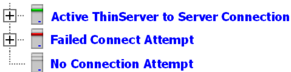
Terminal Server Status Lights
