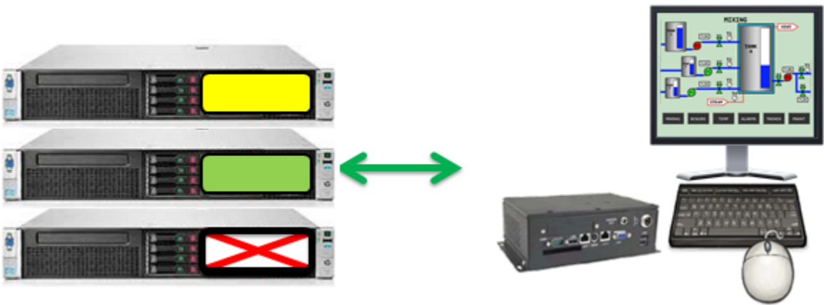
Terminal Connected to Second Terminal Server
